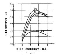
mum conditions for recording on the various kinds of tape. Since the audio input level is the same for all curves, the relative output levels of the various tape types at any particular bias value can be read directly from the curves. The optimum recording bias is approximately that giving the peak output, but in many cases, a somewhat greater bias will give a steadier signal.
